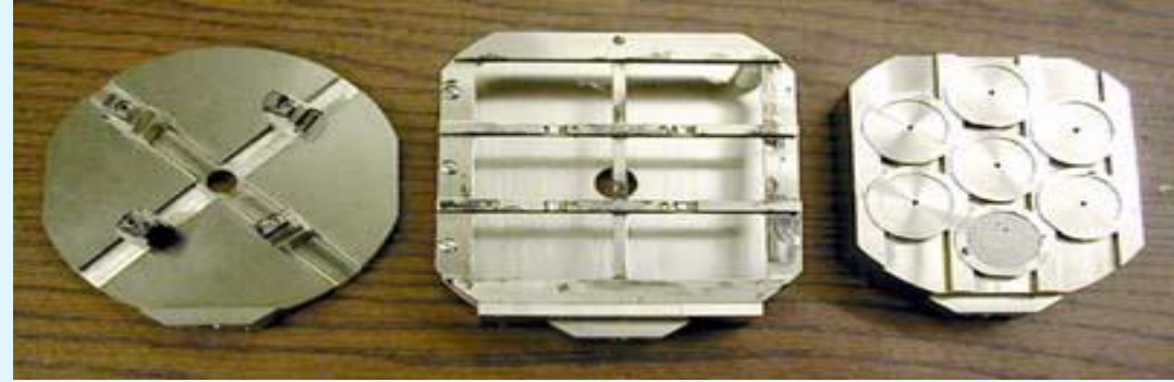
A variety of sample holders can be used for specimen stubs, rectangular sections and round disks; several samples can be loaded at one time in these holders.
